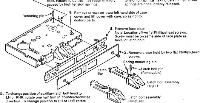
in clockwise direction. Caution: Do not rotate more than 1/2-turn in either direction from factory setting
