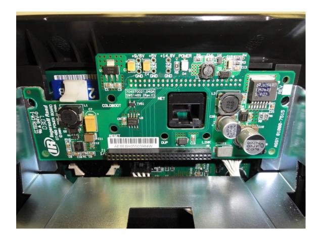
Secure the power board to the unit using the two screws shown in the image below.
