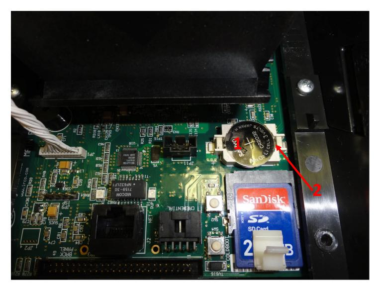
Carefully place the terminal on its top panel so that you are looking at the main board. The lithium battery is located above the SD Card.
