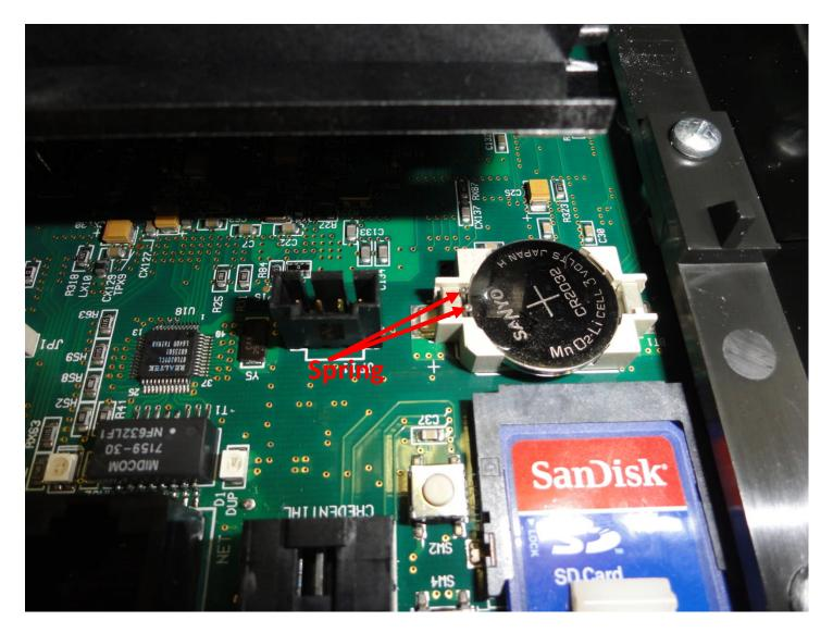
There are two types of battery holder that may be installed on the main board; one with visible spring keeps and one without. The installation of the battery is the same either way. Place the left side of the battery into the battery holder first and snap the battery into place.
