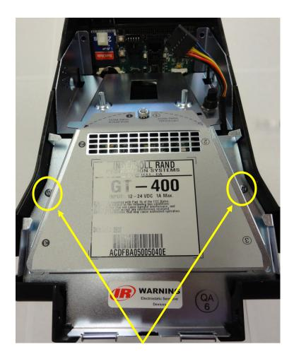
Remove the two screws highlighted and set aside for reuse. Rotate the top of the back plate towards you
