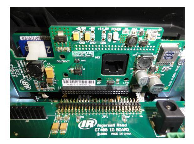
Align the IO's 2 x 25 pin header and connector and gently press them together making sure that it is installed. Secure the IO board to the unit with the screws shown in the image below.
