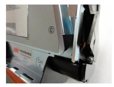
Start with setting the back plate into the battery compartment and start rotating the back plate towards the top. If there is a backup battery installed, make sure that the BB-300 cable is not getting pinched in the lower right hand cable. Stop when you get to the camera cable.
