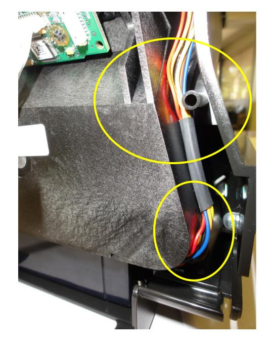
Routing the battery cable if there is a back up battery installed
