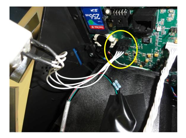
Remove the tamper switch connector from the main board. Do not pull by the wires but depress the tab to release the connector.
