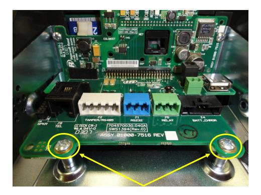
Lay the GT-400 terminal face down of a clean antistatic mat to protect the surface from scratches and the PCBs from ESD damage. Remove the two screws highlighted and set aside for reuse.
