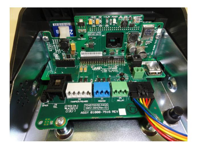
Plugging in the battery backup cable if installed
