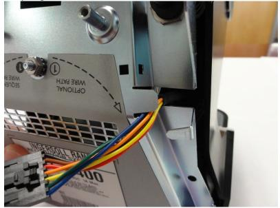
Pull the backup battery cable through the back plate as shown above.
