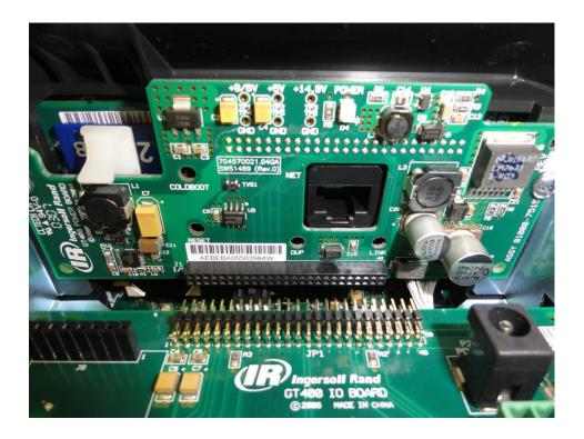
With the terminal still laying face down and while wearing the ESD ground strap hold the IO board by the edges and gently pull the board towards you and set aside.
