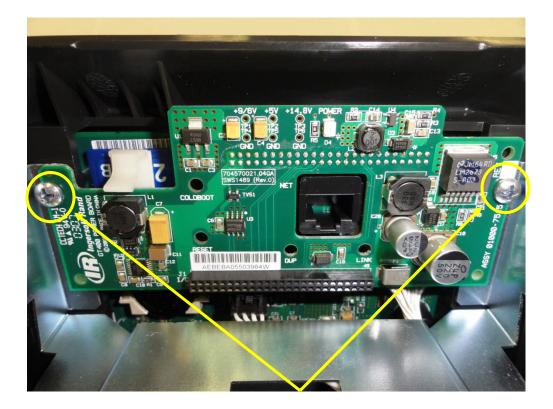
Remove the two screws highlighted and set aside for reuse. Hold the power board by the edges and gently pull the board towards you and set aside.
